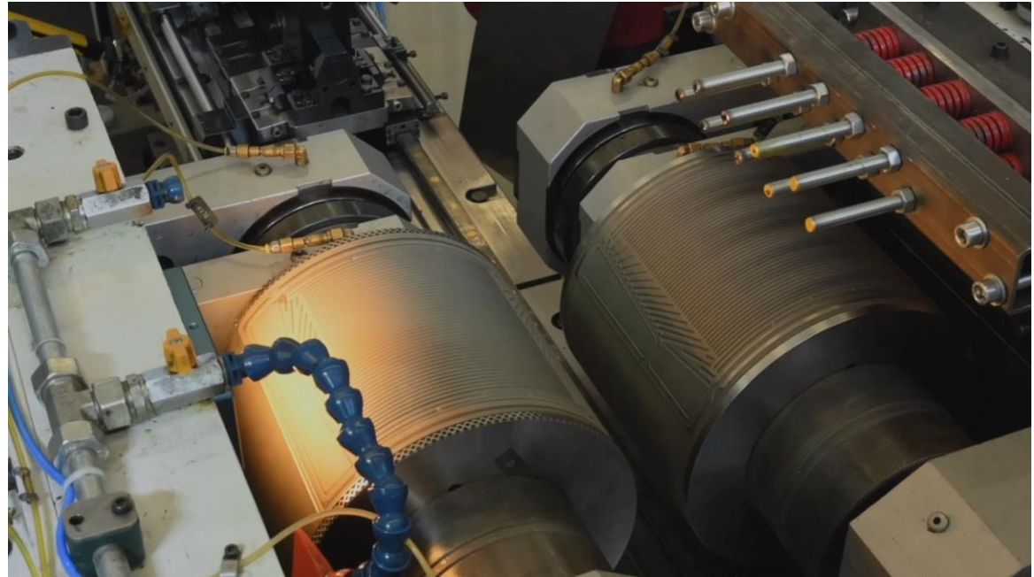
Fig.: Hollow embossing rolling process
