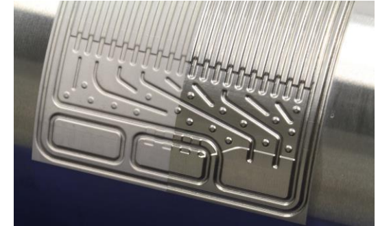
Fig.: Forming roll produced by laser engraving
