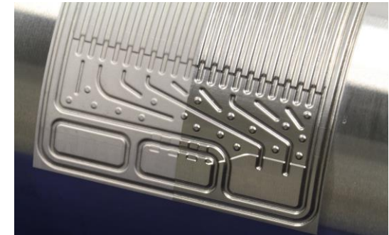
Fig.: Forming roll produced by laser engraving
